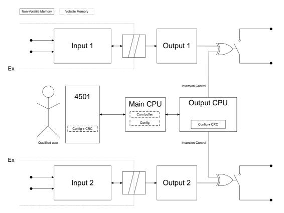
It can be seen, that the complex electronics (Type B) are only used to control the direct / invert setting of the output. The read back of the Output CPU's control signal by the Main CPU for diagnostic purposes and the possible second independent shutdown path are available, but not shown in this diagram.
